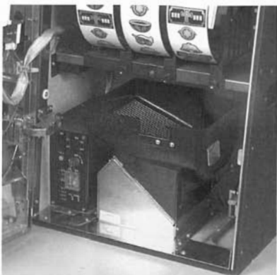
Figure 2: Hopper properly seated in its tracks
